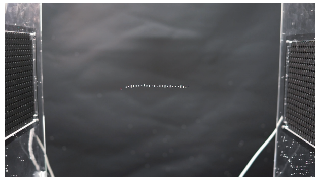
Fig. 1 Levitation by opposed ultrasound phased array.
