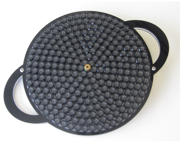
Fig. 1 Prototype of hand-held ultrasonic pollination device.
