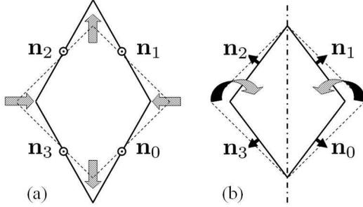
Fig. 4 Assumption about normal vectors. We assume two types of symmetric transformations, (a) squashing and (b) folding.
