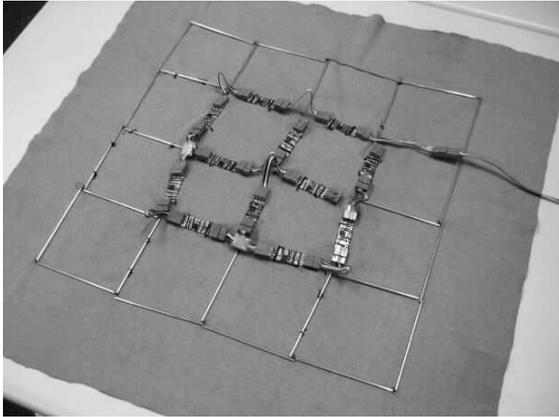
Fig. 10 Prototype of 3DCS (60 × 60 cm<sup>2</sup>). Each link is 10 cm in length. There are the 12 sensor chips.
