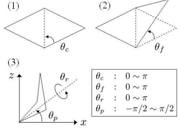
Fig. 5 Procedure of lattice model generation. The corner, fold, roll, and pitch angles are the changing parameters.
