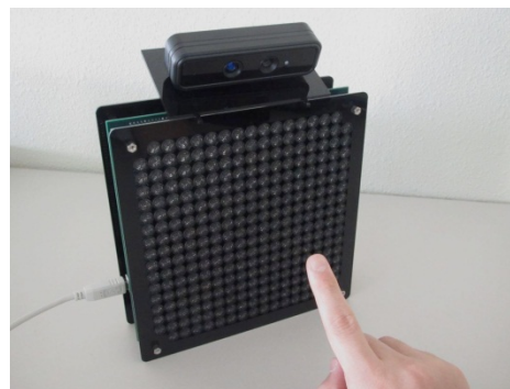
Fig.1 Noncontact tactile display with depth camera.
