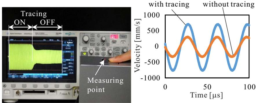
**Fig. 4.** (Left) Overview of experiment, (Right) Vibration velocity of display surface with and without resonance frequency tracing.
