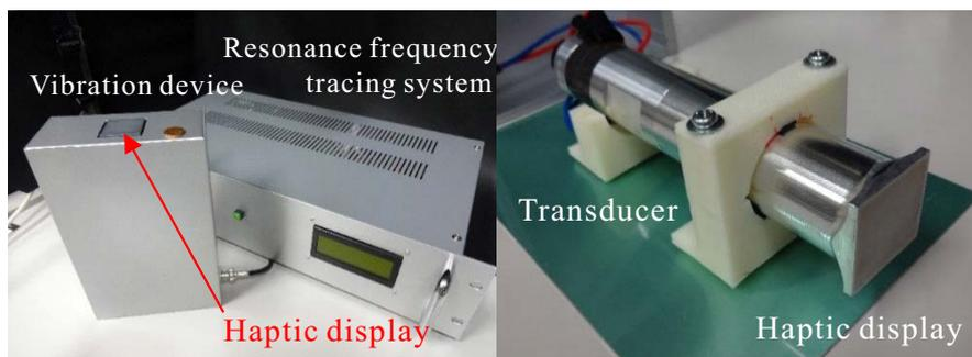
**Fig. 1.** (Left) Overview of Diminished Haptics system, (Right) Structure of vibration device
