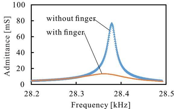
Fig. 2. Admittance of transducer with/without finger
