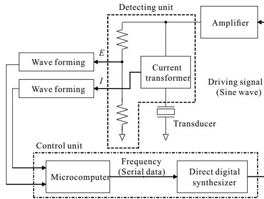
Fig. 3. Diagram of resonance frequency tracing system
