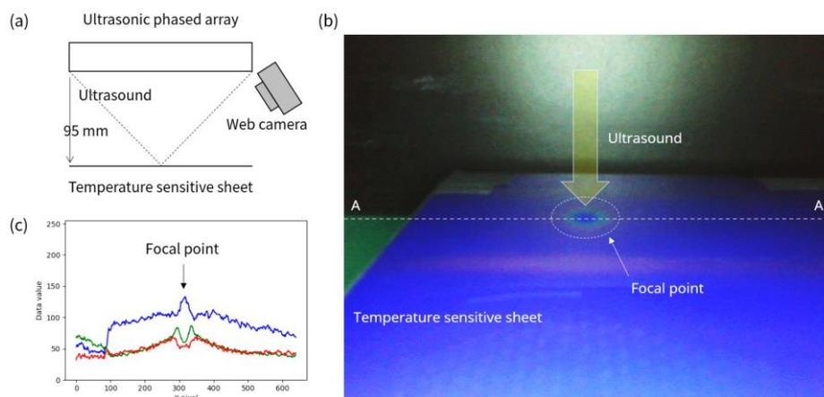
**Fig. 1.** Experiment of visualization of the focal point with a temperature sensitive sheet. The color changes in a few seconds after the ultrasound is applied. (a) Experimental setup. The temperature sensitive sheet was observed with a web camera (640×480 pixel). (b) Image taken by the web camera (note that the brightness and contrast have been modified from the original for ease of viewing). (c) RGB values along the white dotted line A-A' in (b).
